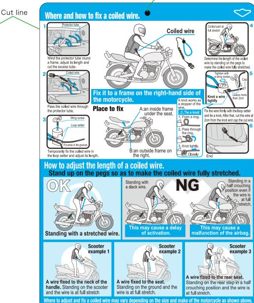
Don't fix a coiled wire to any part where it would disturb
