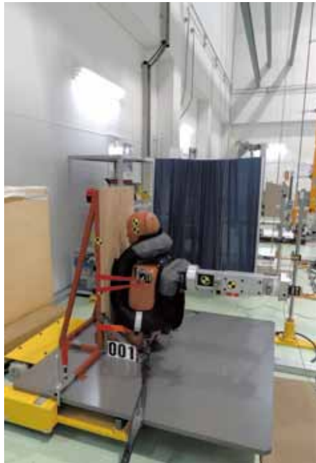
Impact speed : 4.2m/s (15 km/h) Pressure of the airbag : 20 kpa
