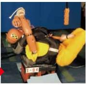
It was found that the airbag reduces the neck acceleration by more than 58% and the body acceleration to 89.4% and effectiveness of the airbag is now verified.
