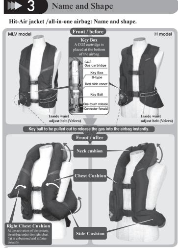
\*2) For a belt adjustment around your waist, pass the belt through belt loops without fail. If the belt is not kept in the belt loops when the system is activated, it may come off and the function of the airbag (shock buffering) may be impaired. \*Although numbers of belt loops vary with models.
