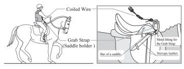
Fix the coiled wire to the center of the grab strap.
