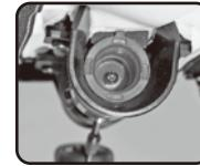
The airbag doesn't work nor inflate if the needle is damaged or deformed.
