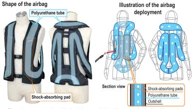
Three-layer construction with the airbag sandwiched between shock-absorbing pads for enhanced shock-absorbing effects.
