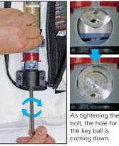
Screw the setting bolt by the hexagon wrench. The metal hole of the key box comes down accordingly.
