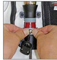
Put the key ball and its metal ring to the metal hole
