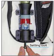
Insert the setting bolt to the bottom of the key box.
