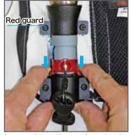
Lower the red guard to check if the key ball is installed correctly. In case the red guard doesn't come down fully, the key ball is not installed correctly.
