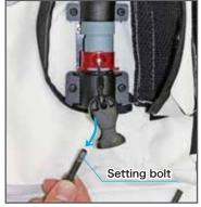
Unscrew the setting bolt and take it away from the bottom of the key box.
