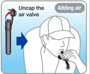
To increase inflation, exhale into the air valve after uncapping it.
