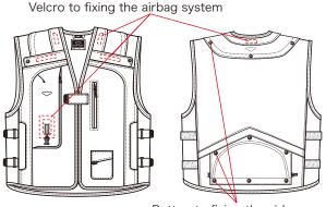
Button to fixing the airbag system
